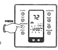
Step 7: Press and release the PROGRAM button until the temperature for the Morning "\_\_\_\_\_" event flashes. Repeat steps 2-4 for the Morning "\_\_\_\_", Day " -\_\_\_", Evening "\_\_\_", and Night " (" events.
